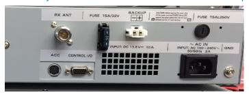
While it is true that the repeaters have a "port" that says "ACC" "and CONTROL I/O" on the rear, and the literature says that the port makes it possible to have an external controller control the repeater, having that come to life in a meaning full way can be challenging, especially when using the repeater in AMS ("Auto-Mode-Select") mode, which basically is what allows the repeater to switch back and forth between analog and digital, and not just be "locked" onto one mode or another.
